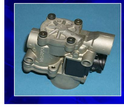
Sends a specific braking pressure to the brake booster controlled by the EBS unit or rear axle modulator during ABS control
