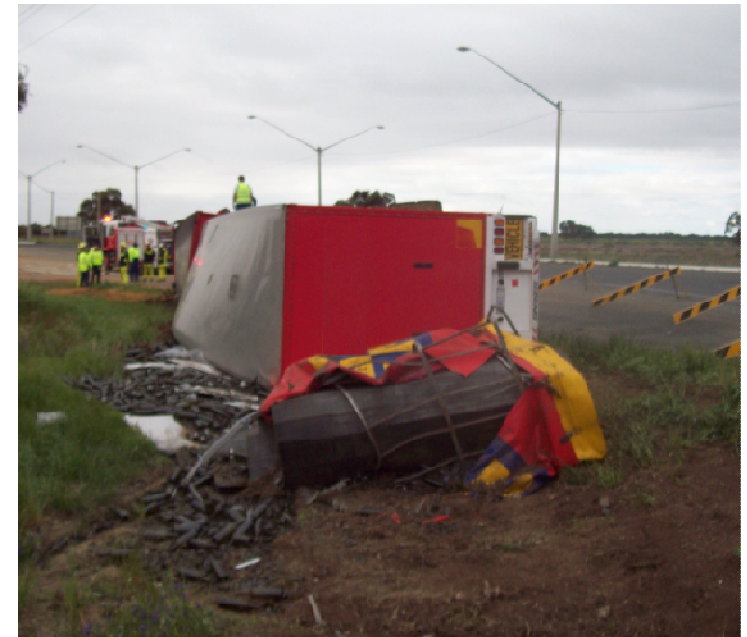
This B-Double rolled over carrying 68,000 empty wine bottles High CoG + ~13 km/hr too fast at country roundabout
