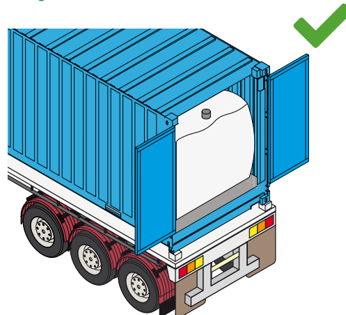
Figure 237 Flexible tank inside container
