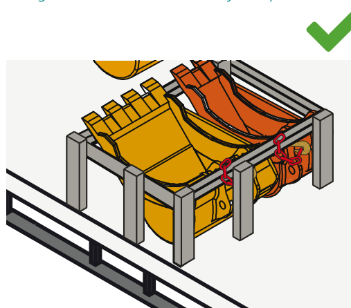
Figure 271 Restraint of auxiliary components
