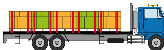
Figure 52 Pallets tied down
