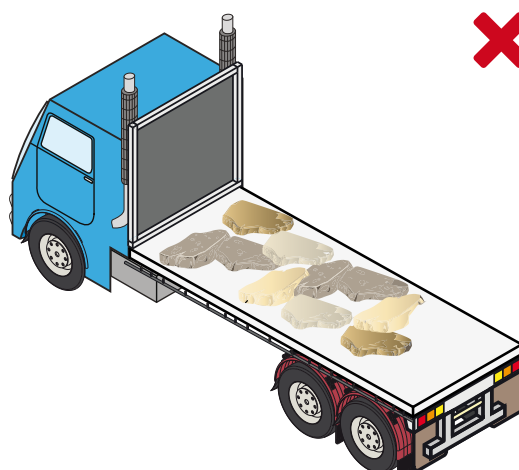
Figure 208 Loose bulk load – no containment
