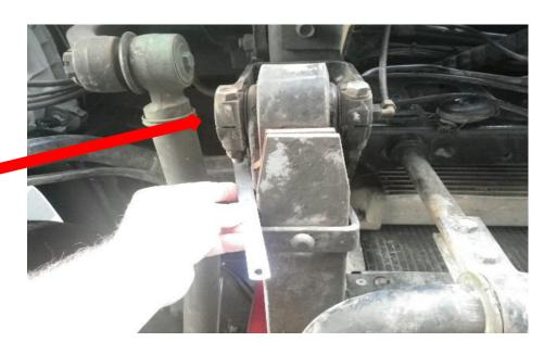
Spring hanger bolts were tightened "finger tight"
